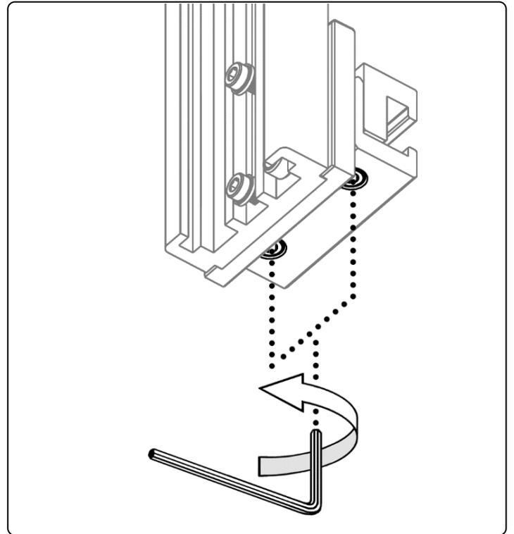
2. Loosen the 2X lower clamp positioning M6 SHSCs on channel so lower clamp can be adjusted within slot on channel.
