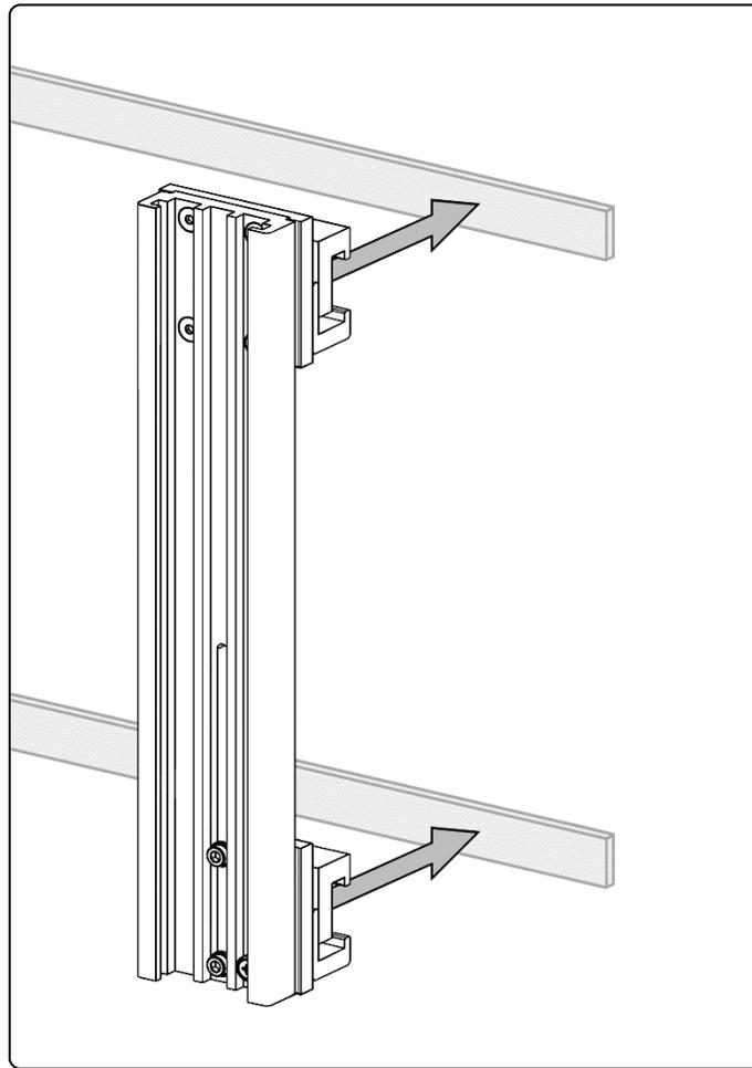
4. Tighten the 2X M6 SHCS on each clamp so the clamps are secure on each rail.
