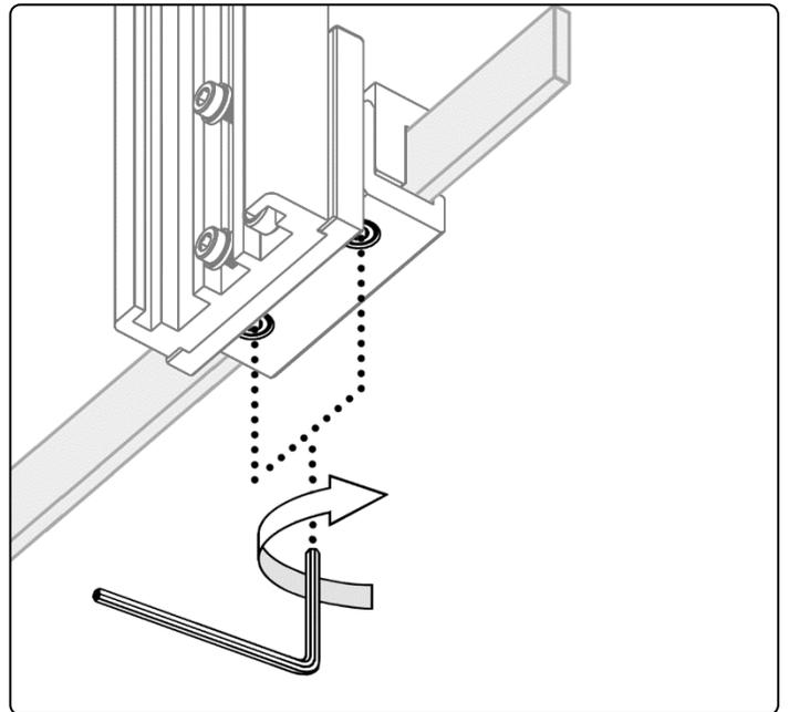
5. Tighten the 2X lower clamp M6 SHCS positioning screws on the channel.
