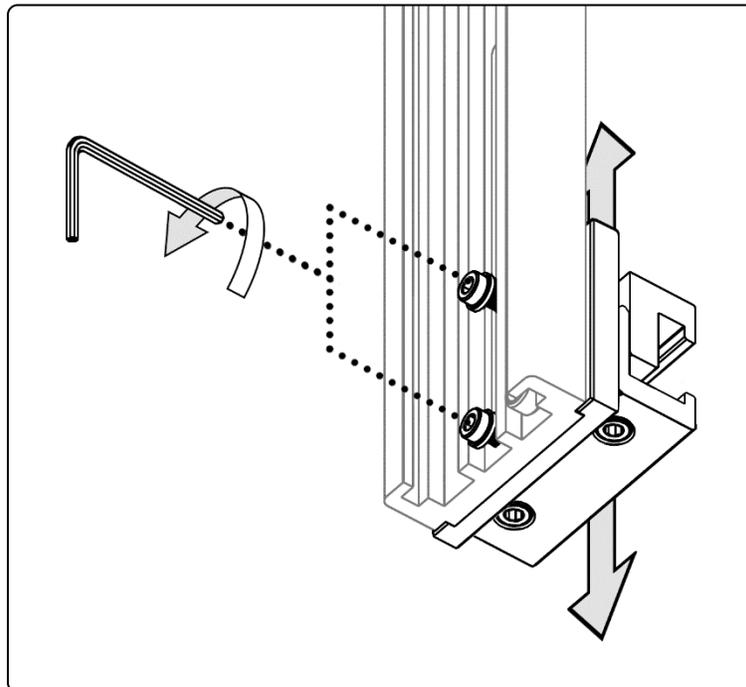
3. Align upper and lower clamps with upper and lower horizontal rails and hang clamps into the rails.
