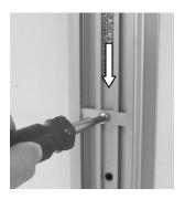
2. Insert Channel Slide(s) into the channel and guide the CPU Mount to the desired height (or top of Adjustable Stop). Using the 1/8" hex wrench provided, tighten socket set screw on each Slide to secure Mount (below right).
