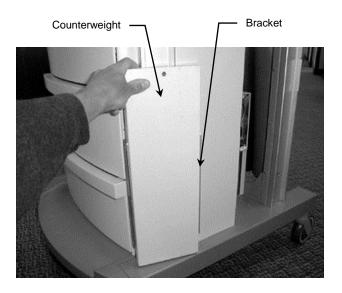
3. Place Counterweight Cover over the Counterweight and Bracket as shown. The two holes on either side should align with the threaded holes in the Bracket. Fasten the Cover to the Bracket using the four (4) #10-32 x 1/4" FHMS provided.
