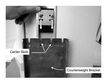
2. Drop the Slide down so the screws engage the Center Slots, install the lower two (2) #10-32 x 5/8" PHMS and tighten all four screws. Place the Counterweight (30lbs/13.6kg) into the Bracket, carefully hold it in place.
