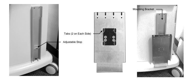
4. Carefully lift Counterweight (30 lbs/13.6 kg) onto bottom lip of Mounting Bracket, holding Counterweight in place (below left). Place Counterweight Cover over Counterweight and Bracket. Align two (2) mounting holes on each side of Cover with corresponding threaded holes in Bracket and fasten Cover to Bracket with four (4) #10-32 x 1/4" FHMS (below right).
