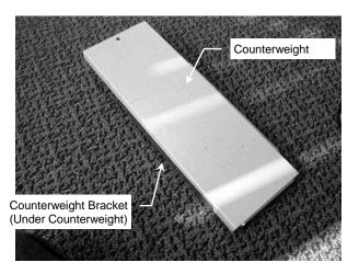
2. Attach Counterweight Cover to Counterweight Bracket with four (4) #10-32 x 1/4" FHMS as shown. Install Counterweight assembly to channel by aligning Slide with channel, then slide the Counterweight into position. Note that the base of the anesthesia machine will support the Counterweight vertically.
