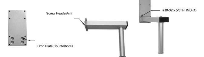
2. Attach Drop Plate to Slide Plate using four (4) #10-32 x 3/4" PHMS (below center and right). Clamp module rack (or other device with clamp) to the Post.
