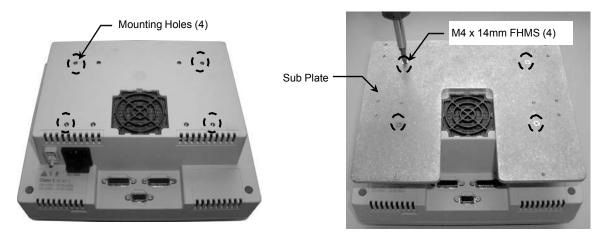
Locate four (4) threaded mounting holes on the Sub plate (below left). Fasten the Sub plate to the display arm with four (4) M4 x 8mm PHMS.
