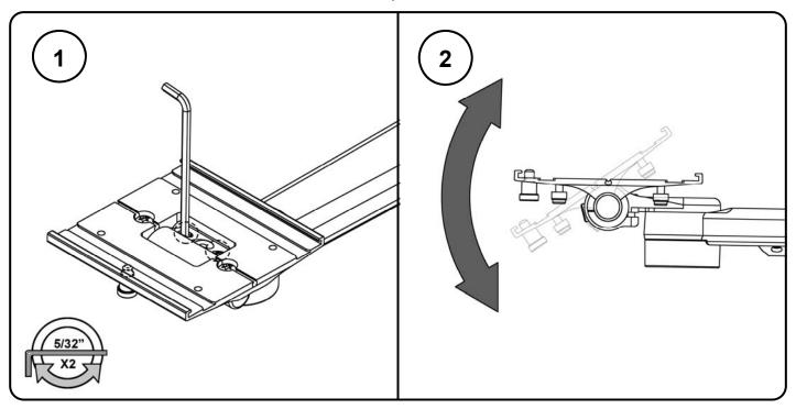
Marning: Tilt tension screws must be torqued to a minimum of 35 in-lbs [4.0 N-m].
