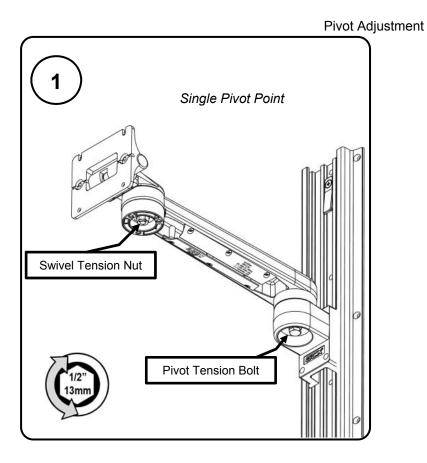
Warning: Swivel tension nut must be torqued to a minimum of 20 in-lbs [2.3 N-m].
