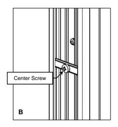
2. Slide Flush Mount into opening at top of channel and position on top of the Adjustable Stop.
