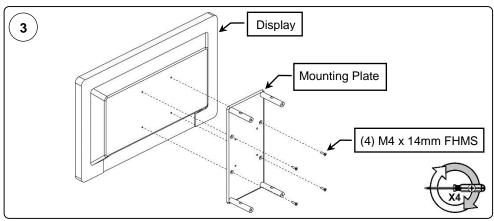
Fasten the HP Thin Client Mounting Plate Assembly onto the Display Mounting Plate Assembly using four (4) 10-32 x 1/2" FHMS.
