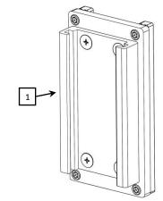
2. Guide Channel to desired height and tighten four (4) M6 x 12 SHCS with M5 hex key (provided).
