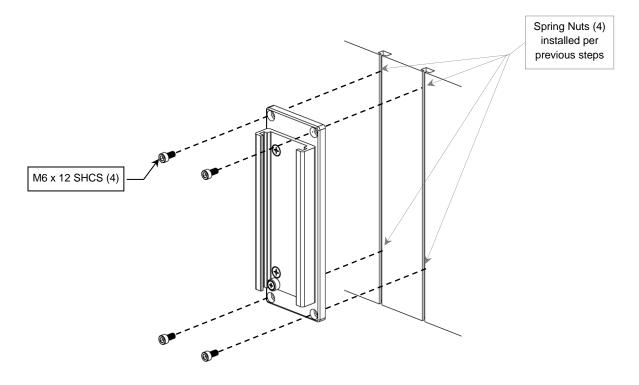
2. Position Channel to desired elevation and tighten four (4) M6 x 12 SHCS with M5 hex key (provided).
