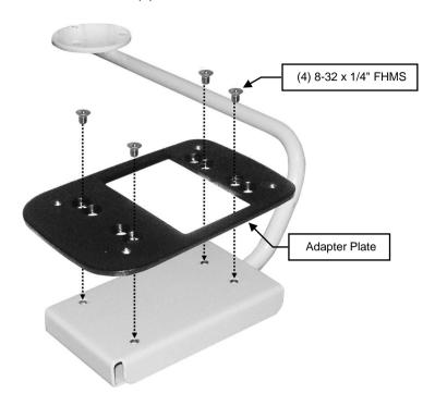
Install Power Cord and USB Cable in to Scanner Base per manufacturer's instructions. Fasten Base to Adapter Plate with (4) Pan Head screws included with the Adapter.
