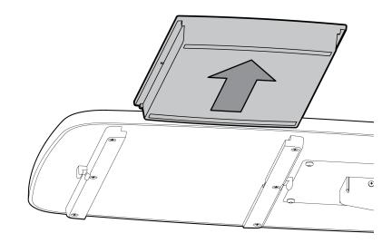
1. To reinstall the drawer, slide the Drawer back into the rails and close the drawer.
