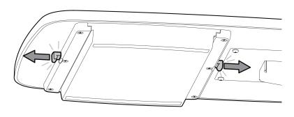
2. Once the Latches are unlocked, simply slide the Drawer completely out of the rails.
