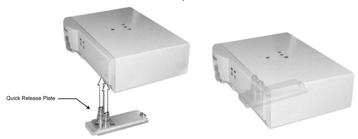
2. Slide the mounted G5 assembly into the channel from the rear of the stack mount. Pull Plunger Pin up while sliding G5 into channel. Release Plunger Pin into Clearance Hole to lock into place.
