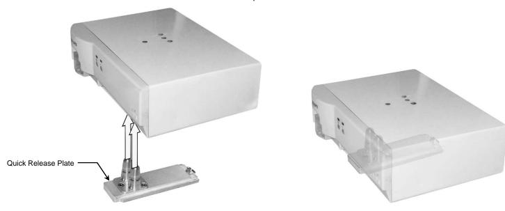
2. Slide the mounted G5 assembly into the channel from the rear of the stack mount. Pull Plunger Pin up while sliding G5 into channel. Release Plunger Pin into Clearance Hole to lock into place.
