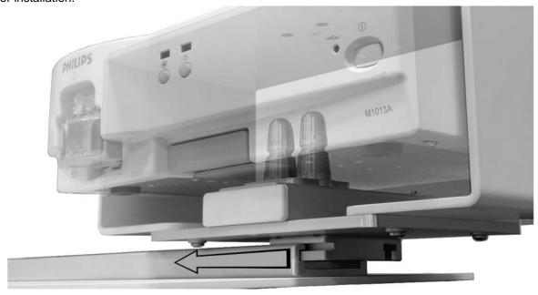
2. To fasten horizontal mount, tighten (2) 8-32 x 5/8" PHMS with a Philips screwdriver.
