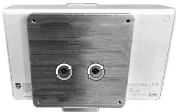
2. Thread two (2) M4 X 10mm PHMS into the top two (2) threaded holes of the VESA mounting pattern located on the back of the adaptor, leaving 4mm of thread exposed.
