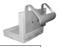
Use two (2) M4 x 12mm PHMS when mounting Bed Hook to a Docking Station with Battery Extension.
