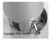
2. Align two (2) mounting holes in Foot Pedal Assembly with two (2) threaded mounting holes in bottom of Post, ensuring that Foot Pedal is positioned between two legs of the Base. Using the 3/16" hex key (provided), fasten Pedal Assembly to Post with two (2) 1/4-20 x 3/4" SHCS.
