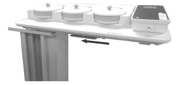
4. Fasten the device by pulling the Plunger on the Slide-In Mounting Plate and releasing when the device is in place.
