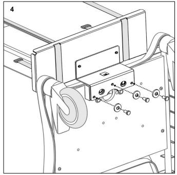
Using a 1/2" socket wrench, secure the tray assembly to the base spacer with (3)  $5/16-18 \times 5/8$ " bolts and (3) washers.
