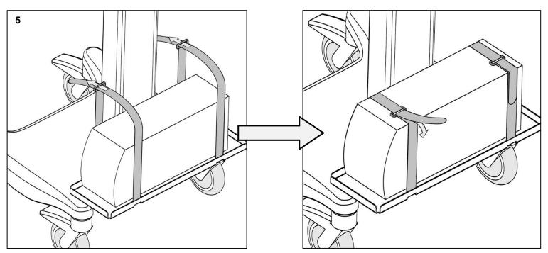
Install UPS to tray, and secure with the (2) Velcro straps.
