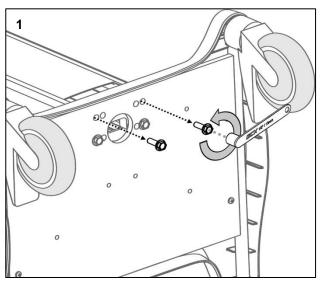
Lay cart down so bottom of cart base can be accessed. Remove and discard the (2) rear column flange bolts with a 1/2" socket wrench.
