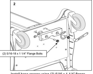
Install base spacer using (2)  $5/16 \times 1 1/4$ " flange bolts.
