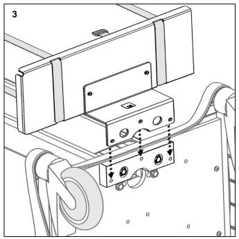
Align the (3) mounting holes on the tray assembly with the corresponding (3) threaded mounting holes on the base spacer.
