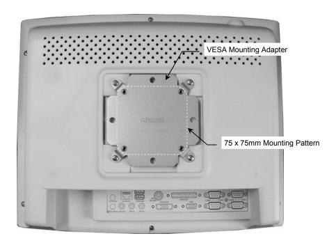
2. Fasten the display to the L-Bracket (upper 75 x 75mm mounting pattern) with four (4) M4 x 10mm PHMS.
