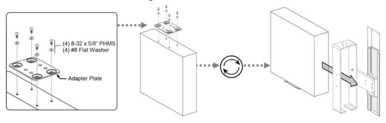
2. Align the (4) mounting holes on the Flush Mount with the (4) threaded mounting holes on the adapter plate. Using a Philips screwdriver, secure the module housing with (4) 8-32 x ¼" FHMS as shown below.
