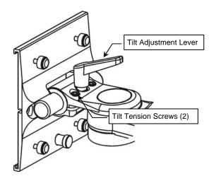
**Installation Note:** The Tilt Adjustment Lever is a multi-position clamping lever that operates by lifting, rotating, and releasing the handle.
