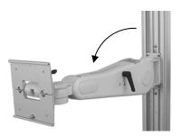
CAUTION: The Utility Hook must be rotated to the side, or removed, if the VHM Arm is raised above the parallel position shown below right.
