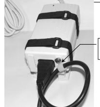
**3.** Connect power supply cord and insert cord in cable restraint as shown.
