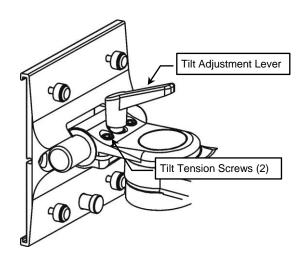
**Installation Note:** The Tilt Adjustment Lever is a multi-position clamping lever that operates by lifting, rotating, and releasing the handle.
