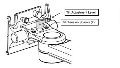
**Installation Note:** The Tilt Adjustment Lever is a multi-position clamping lever that operates by lifting, rotating, and releasing the handle.
