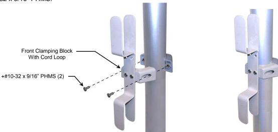
2. Fasten Power Strip Adaptor Plate to to Front Clamping Block with two (2) # 10 x 5/8 (FHSMS).
