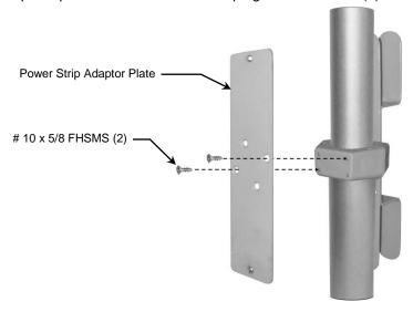
**Installation Note:** The Outlet Strip may be mounted horizontally or vertically on the roll stand post. Select the orientation that best suits your application and follow the procedure below:
