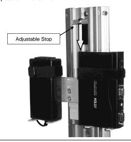
2. Guide the Channel Slide on the back of the Power Supply Cover into the top of the channel and lower the assembly down on to the Adjustable Stop.
