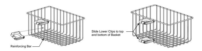
3. Slide Clips over the open end of the post. Position Basket at desired height and install two (2) #8-32 pan head machine screws (PHMS) and #8-32 hex nuts as shown below. Tighten screws until Basket does not rotate on post.
