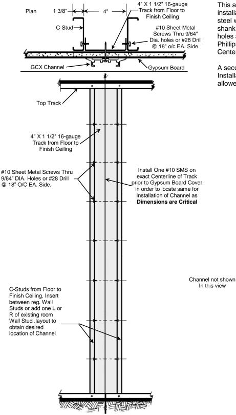
This anchorage will allow for a quick and simple installation of the Standard Wall Channel. 16-gauge steel will prevent the material from extruding up the shank of the screw (Stripping). 11/64" diameter holes are required for #12 X 2-3/4" High Tensile, Phillips Head Screws (4) installed down the Centerline (Non-Seismic Applications).
