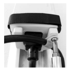
Secure Power Cable with Retainer
