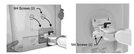
**"Slide-on" Type:** Pull the Plunger at the front of the Mounting Plate. Slide the instrument Mounting Adapter into the Mounting Plate until the Plunger snaps into the clearance hole in the Adapter. Tighten the Nylon screws on the rear or underside of the Plate.
