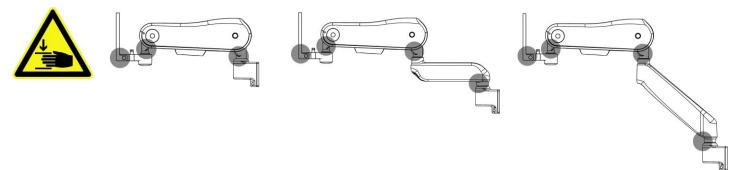
Remove the keyboard and/or keyboard tray only when the VHM-25 Arm is at the highest position. Due to the counter balance function, the VHM-25 Arm may naturally rise to the highest position when weight is removed. This can happen suddenly if the weight is removed at any height other than the highest point.
