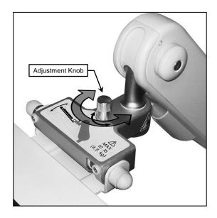
6.4 Folding Tension Adjustment – If the keyboard tray becomes difficult to fold up into the vertical position, or will not maintain the folded up position, then adjust the folding tension. Start by removing both protective caps covering the Folding Tension Adjustment Bolt. Using a 1/2" (13mm) wrench on each end of the bolt and nut assembly, tighten or loosen the Folding Tension Adjustment Bolt until the desired Folding Tension is achieved. Replace the protective caps when done.
