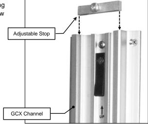
**4.2** While supporting the bottom of the VHM-25 Arm, guide the Slide into the top of the Channel (right) and position it so there is a <sup>3</sup>/<sub>4</sub>" gap between the Slide and Adjustable Stop.
