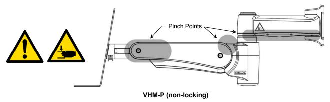
Remove the Device only when the Arm is at the highest position. Due to the counter balance function, the Arm will naturally rise to the highest position when weight is removed. This can happen suddenly if the weight is removed at any height other than the highest point.
