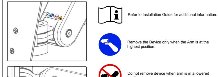
Do not remove device when arm is in a lowered position.
