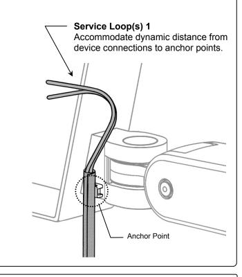
Anchor Cable Bundles. After Service Loop 1 is determined adjust the Cable Sleeve and secure each cable bundle to a Cable Anchor using a cable tie around 1/2" (13mm) from the end of the Cable Sleeve. Before securing the cable tie, ensure the service loop to the device is still correct and secure only one bundle per anchor.
