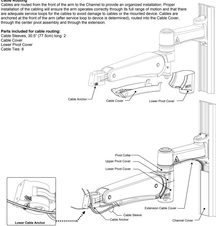
Three (3) Cable Anchors are provided at the front of the arm to secure cables and create the correct service loop. Cables are secured to the anchor points using plastic cable ties included with the Arm. If replacement cable ties are required, standard commercial cable ties can be used.
