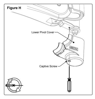
After the Lower Pivot Cover has been installed, move the arm through its entire range of motion. Make sure device cables do not bind or restrict the movement of the arm, and are clear of potential pinch points that may damage the cables.
