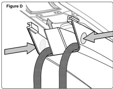
Rotate the pivot collar so that the gap is positioned in line with the seam in the Upper Pivot Cover. Spread the Upper Pivot Cover at the seam and guide the cable sleeve / cable bundle upwards past the pivot collar and into the extension Cable Cover opening – **Figure E**. Feed the cable sleeve / cable bundle through the extension to the channel – **Figure F**.
