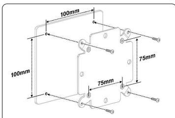
Displays with a  $100 \times 100 \text{mm}$  mounting pattern require attachment of the 75 to 100 mm VESA Mounting Adapter to the display.
