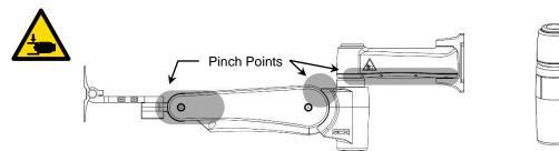
• Remove the Device only when the Arm is at the highest position. Due to the counter balance function, the Arm will naturally rise to the highest position when weight is removed. This can happen suddenly if the weight is removed at any height other than the highest point.
