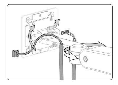
Anchor Cable Bundles. After Service Loop 1 is determined adjust the Cable Sleeve and secure each cable bundle to a Cable Anchor using a cable tie around 1/2" (13mm) from the end of the Cable Sleeve. Before securing the cable tie, ensure the service loop to the device is still correct and secure only one bundle per anchor.
