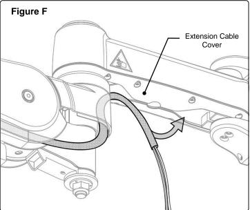
The end of the Cable Sleeve or marked Cable Bundle should be approximately 1.5"-3.5" (38-89mm) inside the Extension Cable Cover – **Figure G**. Align the captive screw with the threaded mounting hole under the center pivot assembly and secure with a #2 Phillips screw driver. Do not overtighten the screw – **Figure H**.
