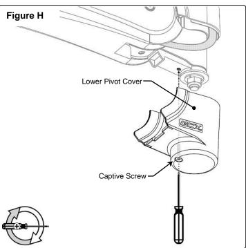
After the Lower Pivot Cover has been installed, move the arm through its entire range of motion. Make sure device cables do not bind or restrict the movement of the arm, and are clear of potential pinch points that may damage the cables.
