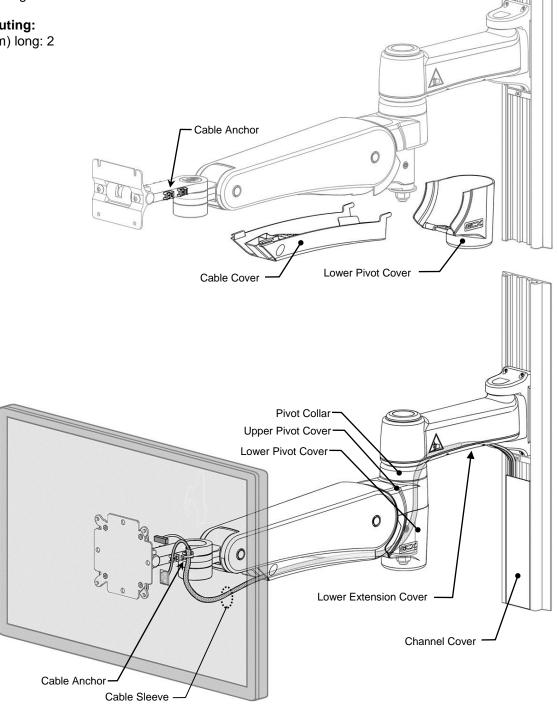
Four (4) Cable Anchors are provided at the front of the arm to secure cables and create the correct service loop. Cables are secured to the anchor points using plastic cable ties included with the Arm. If replacement cable ties are required, standard commercial cable ties can be used.
