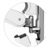
ENCLOSED CABLES AND PIVOT POINTS
